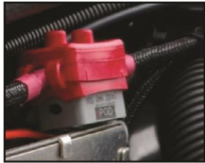
Auto reset circuit breaker
