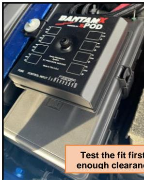
Test the fit first to be sure there is enough clearance and easy access.
