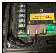
Before installing onto the fender, run cable up through the slot from the bottom. Plug the cable into either port. Adjust the cable to ensure the cover will close properly.
