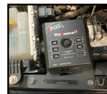
Align slots over threaded holes and align bracket parallel to fender and tighten both bolts.
