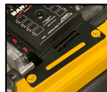
Align slots over threaded holes and align bracket parallel to fender and tighten both bolts.
