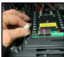
Before installing onto the fender, run cable up through the slot from the bottom. Plug the cable into either port. Adjust the cable to ensure the cover will close properly.
