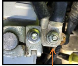
Negative side – 12mm socket
