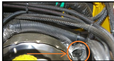
Look on right side of brake boost for pass through
