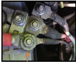
Positive side – 10mm socket
