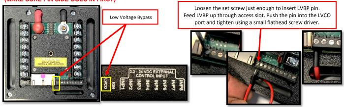
3. Remove red cap & 3/8 nut from positive battery cable terminal.
