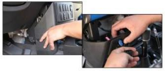
• Route the wire harness from the source through the existing hole in the firewall. Then route underneath the steering column and through the side of the switch panel housing.
