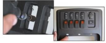
• Connect harness to switches (see switch connection diagram return switch panel to the center console and route longer pigtail up to the switches next to the steering column.
