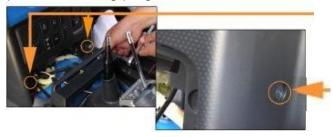
• Temporarily replace the transfer case knob to protect switch panel from scratches. Gently remove switch panel. Make sure to label and disconnect existing factory switches.
