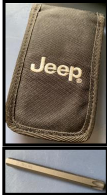
T-40 TORX bit from the Jeep tool kit
