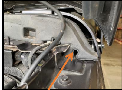
Pass cable through here
