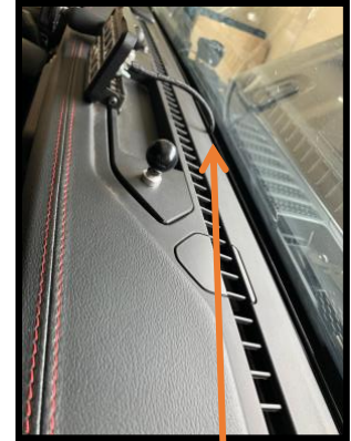
Pass cable through windshield threshold
