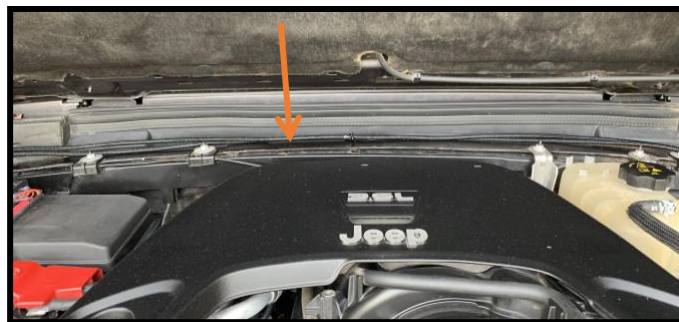
Place bracket over holes. Reuse the bolts and tighten. Leave far right hole open.
