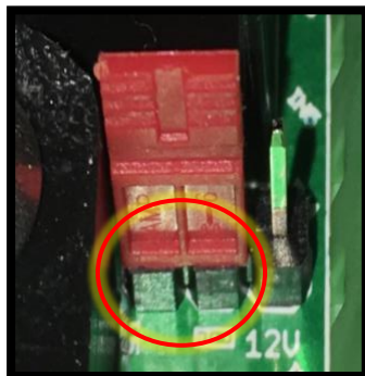
JUMPER ON 2 PINS ON LEFT FOR GROUND TRIGGER
