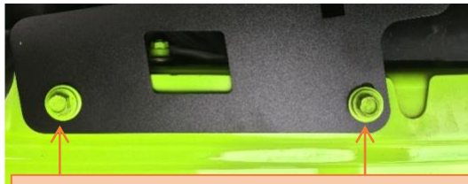
Place plate over holes. Install both bolts and tighten.
