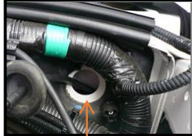
Use this grommet on upper right side of brake booster
