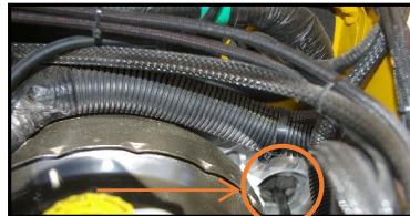
Look on right side of brake booster for pass through
