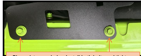
Place plate over holes. Install both bolts and tighten.
