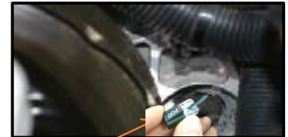
Pull plug through gently by the cable and not the plug
